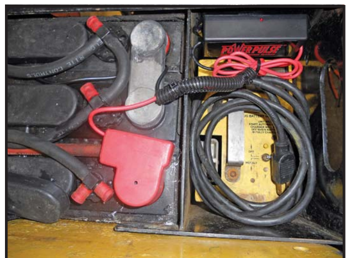
One PP-36-L can be used to maintain three 12V batteries in series or a PP-12-L can be connected to each 12V battery.
